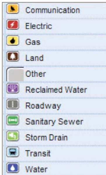
Facility Types in Envista conform to industry-standard colors for One-Call systems. For example, orange is communications, red is electricity, yellow is gas.
